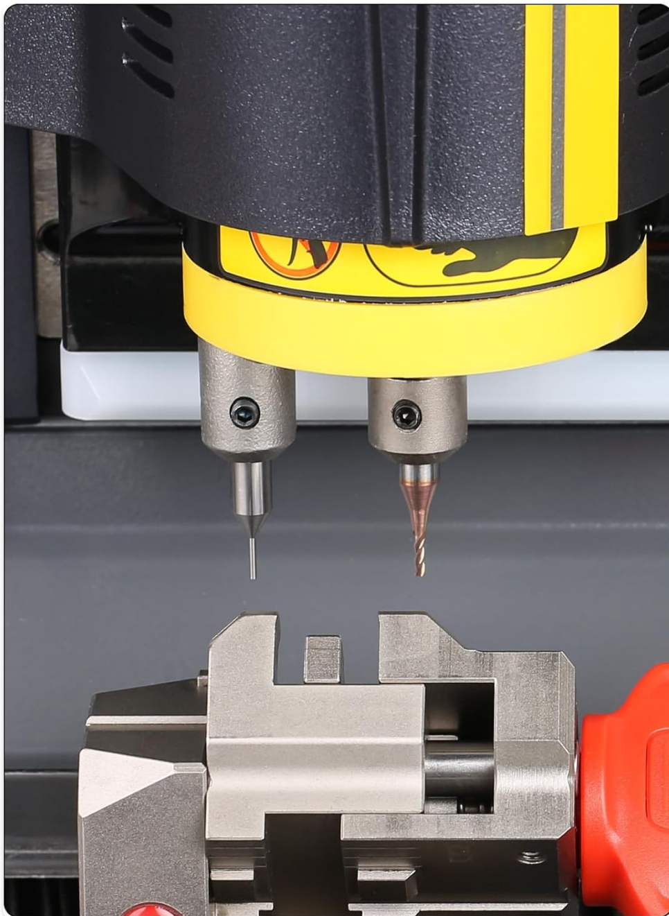
Image: The 1.5mm milling cutter correctly installed in an Xhorse key cutting machine, positioned alongside the machine's probe, demonstrating readiness for key cutting operations.
