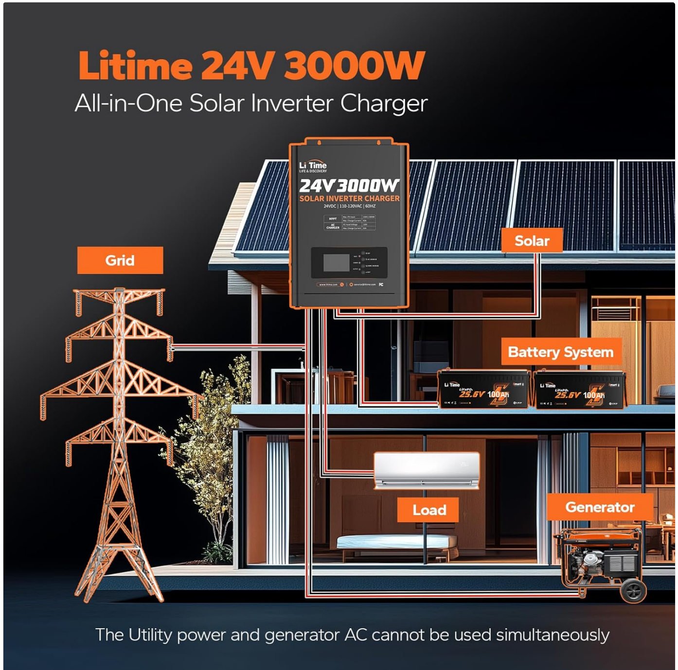
Figure 5.1: Typical system connection diagram for the LiTime Solar Inverter Charger.
