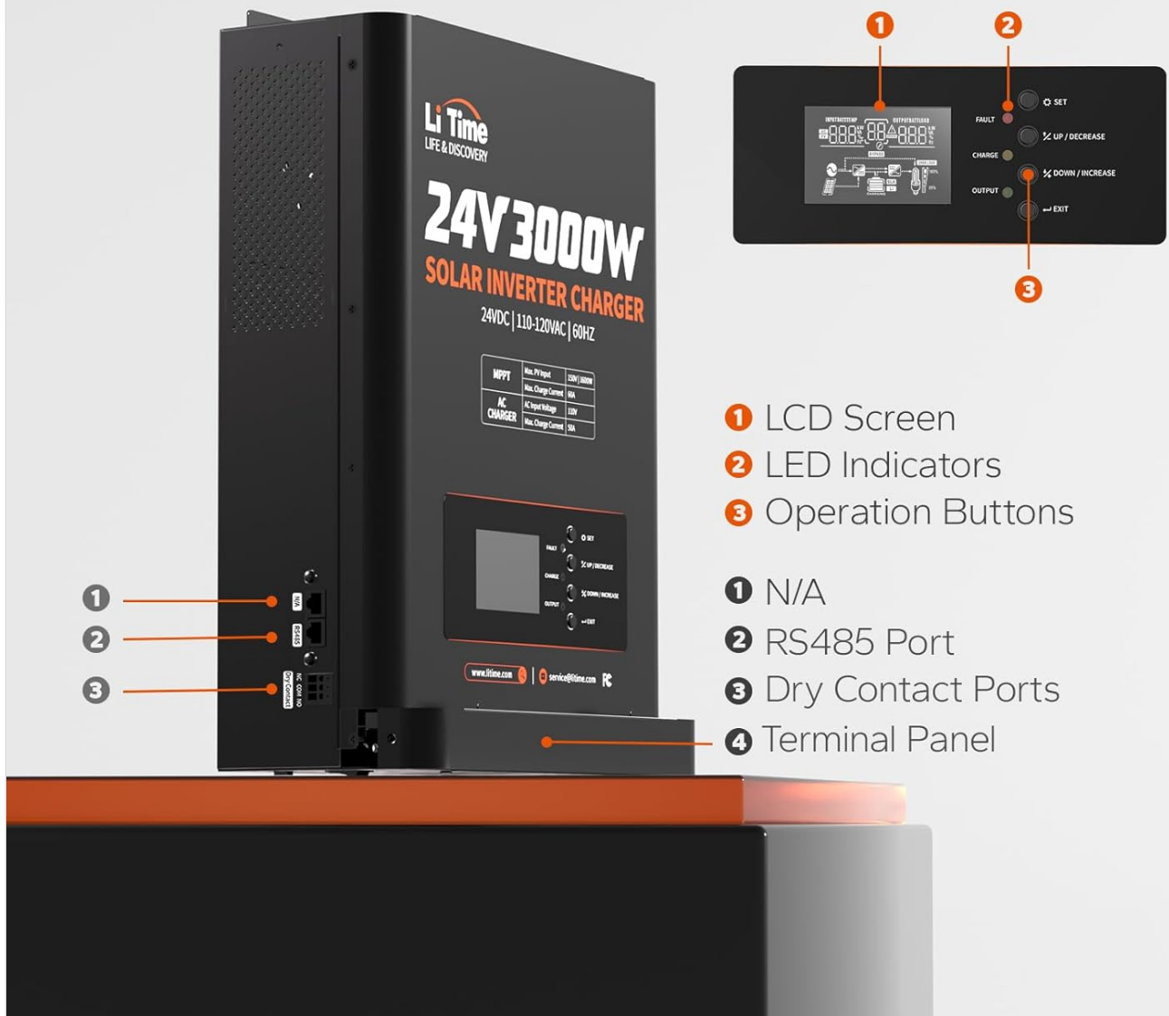
Figure 4.1: Physical components of the inverter charger.
