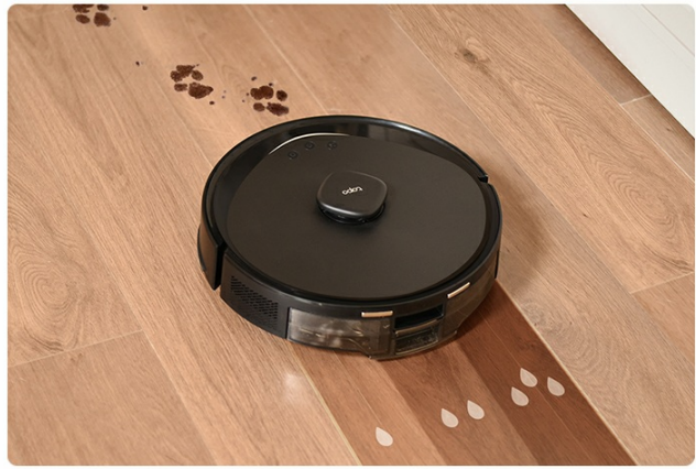
Figure 6.7: The robot vacuum intelligently avoiding carpeted areas while in mopping mode to prevent wetting.
