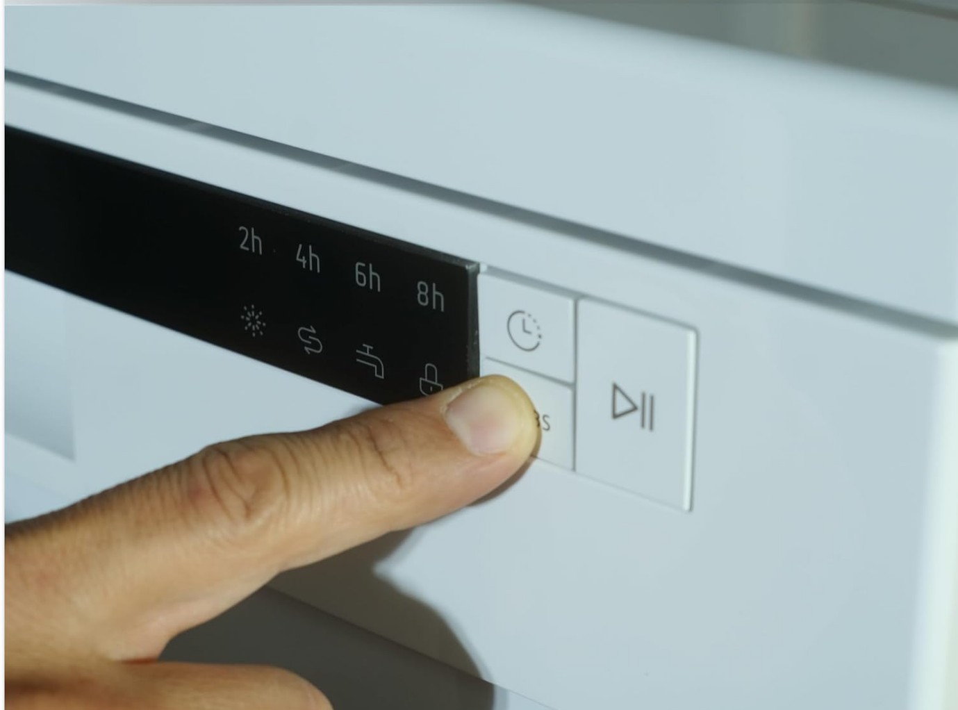
Image 5: A hand interacting with the control panel of the dishwasher. This close-up shows the LED indicators and push-button controls for selecting programs and functions like delayed start and half load.
