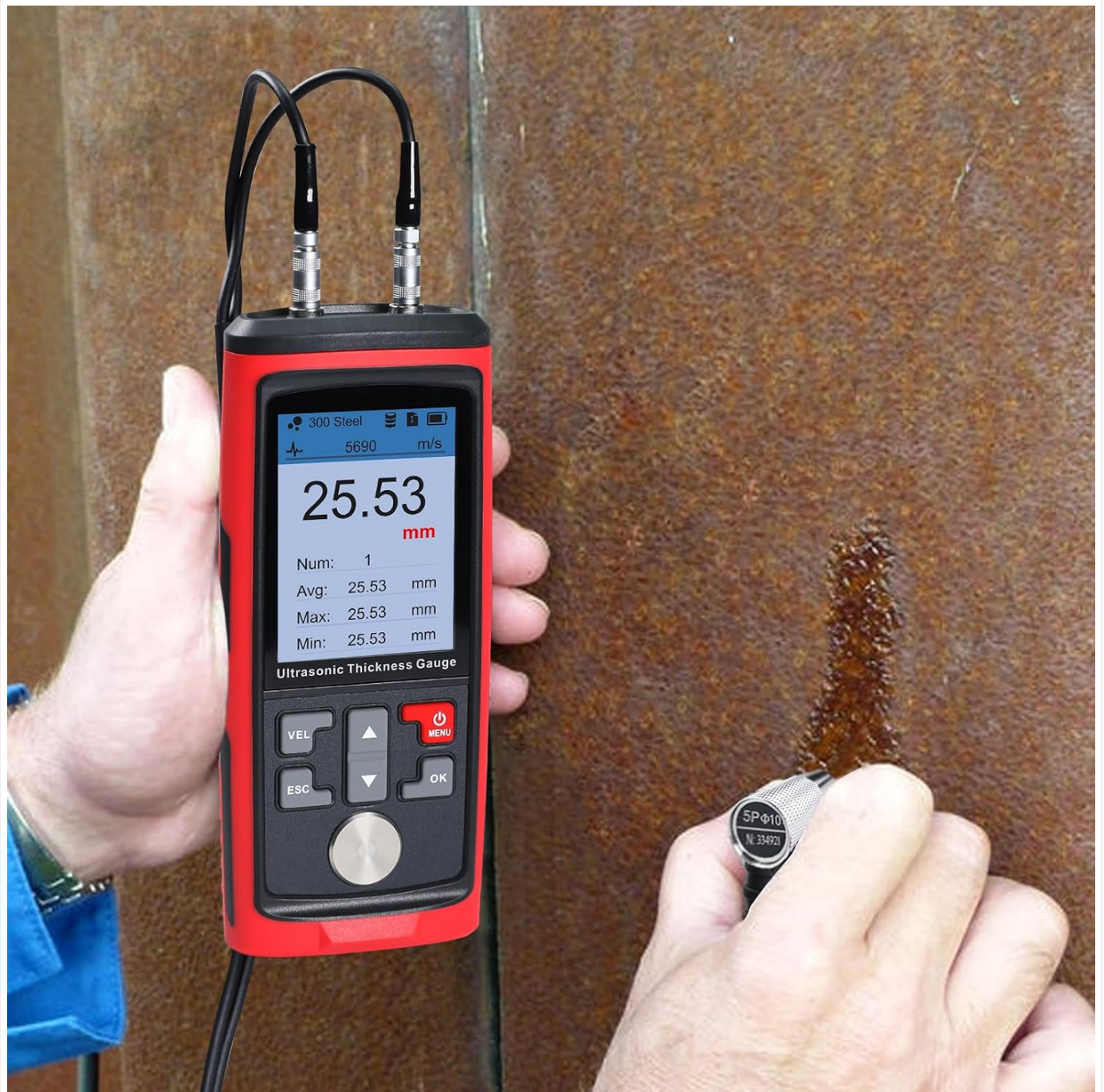
Image: A user holding the thickness gauge and probe against a large metal surface to take a measurement.
