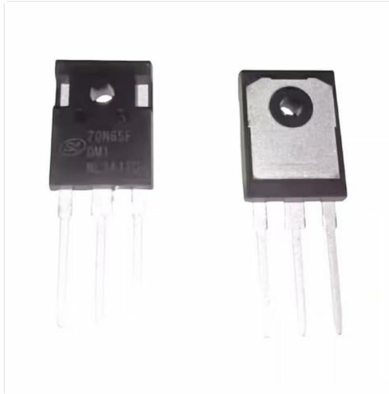
This image displays the SGT70N65FDM1 power transistor, typically housed in a TO-247 package, showing its three leads and heat sink tab. The TO-247 package is designed for high power dissipation.
