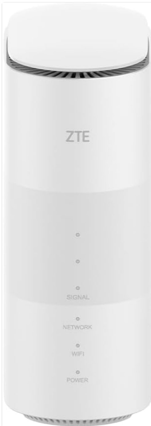
Figure 2: Close-up of the ZTE G5B front panel, highlighting the LED indicators.
