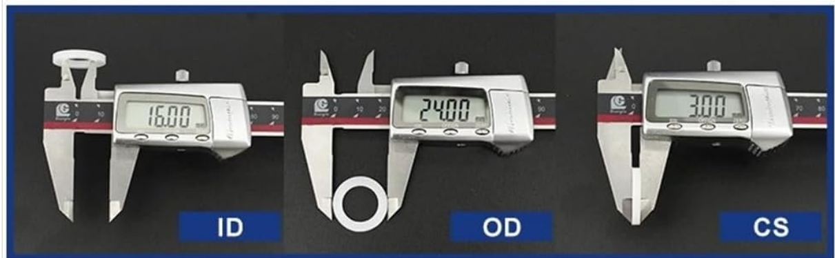
Image 3: A visual guide demonstrating how to measure the Inner Diameter (ID), Outer Diameter (OD), and Cross-Section (CS) of a gasket using digital calipers.
