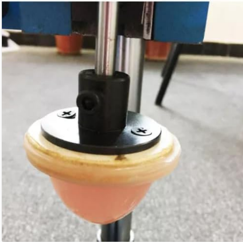
Image 5.3: Detailed view of the printing pad and its mounting.
