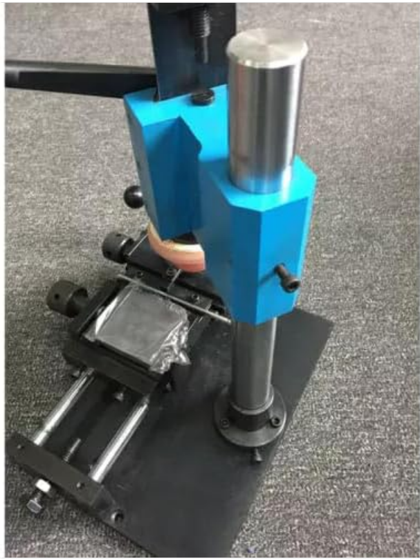
Image 5.1: The machine during the ink transfer phase, showing the ink plate.
