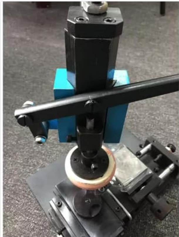
Image 5.2: Close-up of the printing pad making contact with the ink plate.
