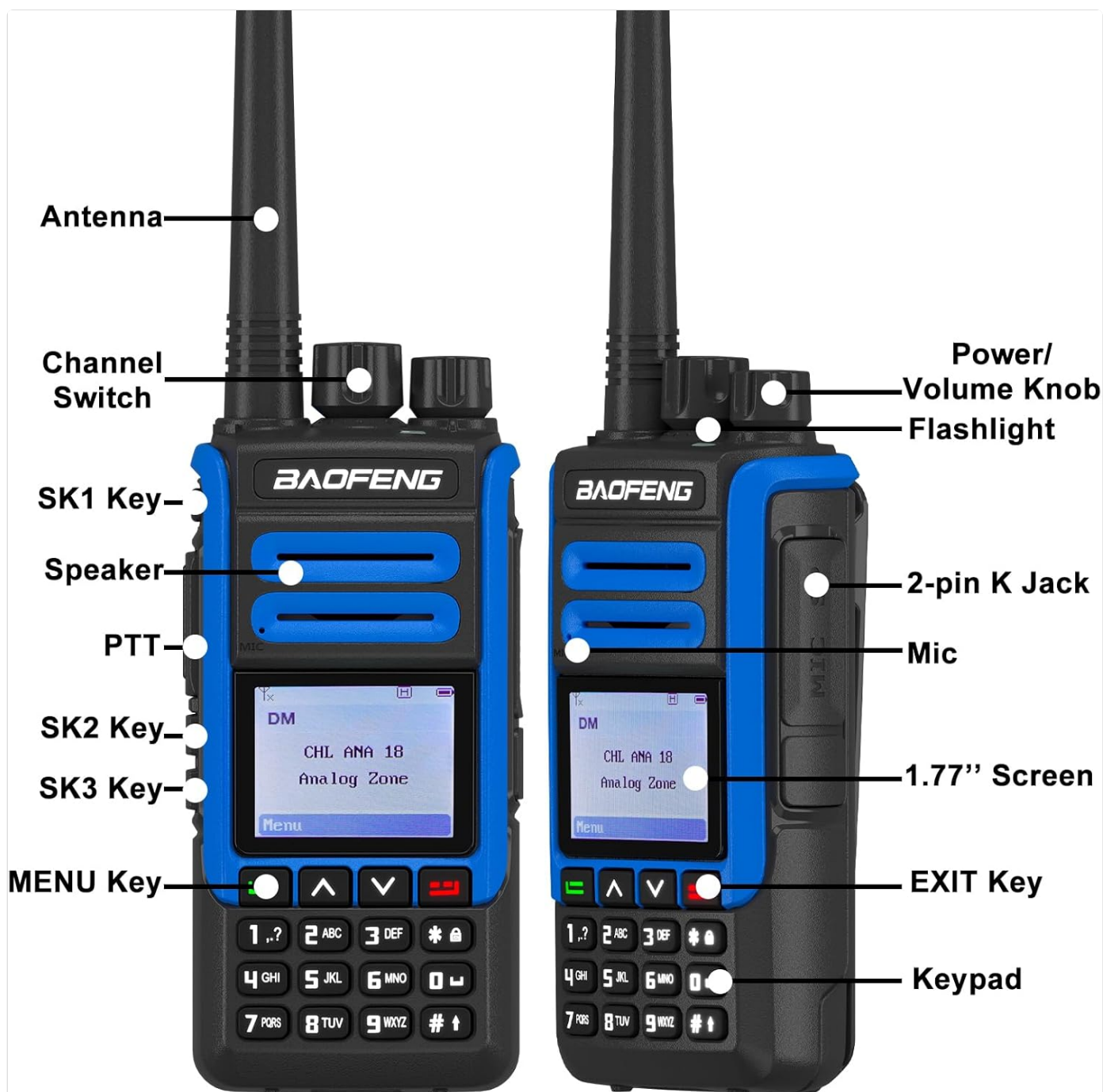
Figure 2: Labeled diagram of the BAOFENG DR-1802U radio, highlighting the 2-pin K Jack for accessories.
