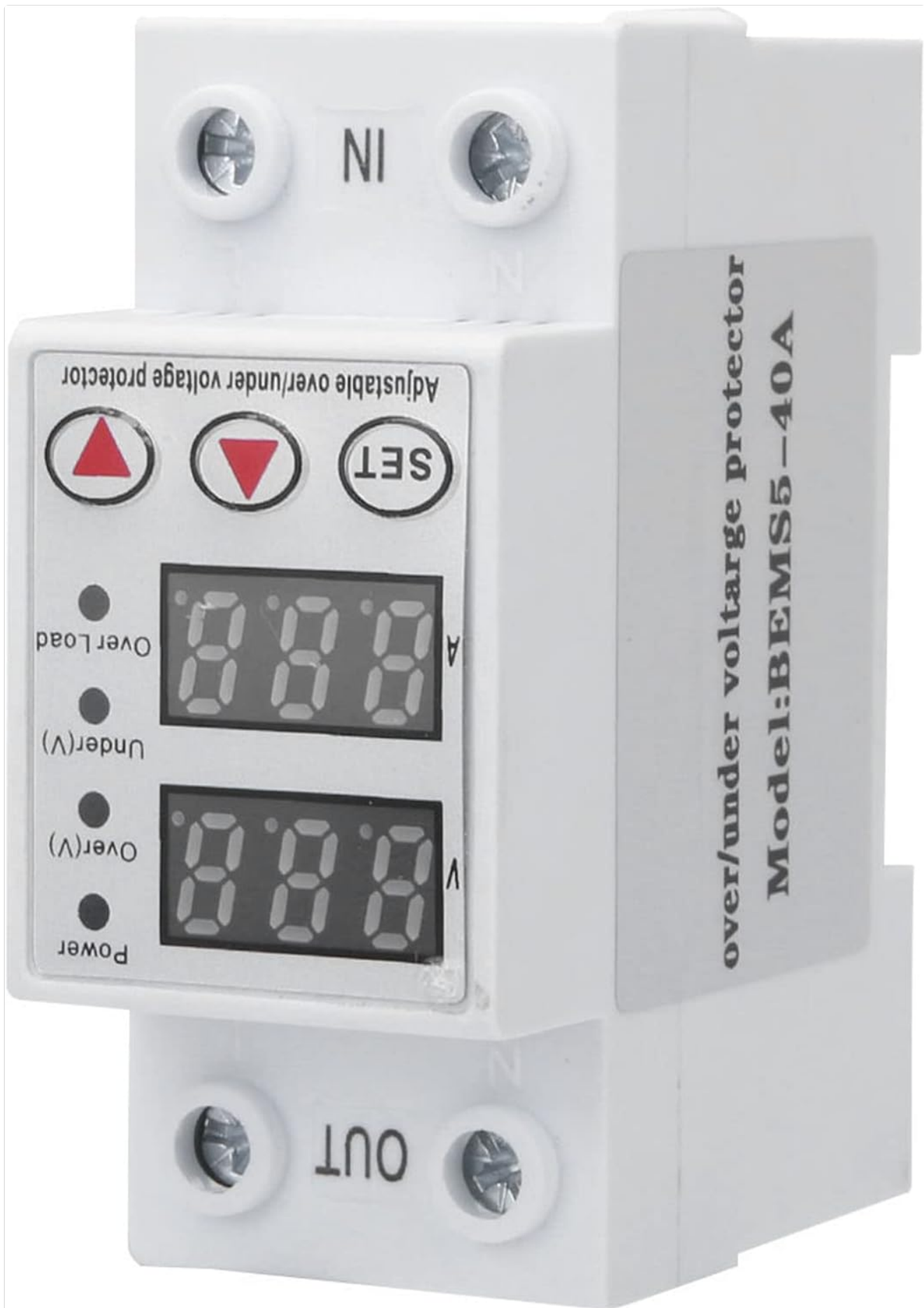
Figure 6.1: Front view of the ASHATA BEMS5-40A Digital Voltage Protector. The device features an LCD screen displaying voltage and current, along with 'SET' and arrow buttons for parameter adjustment. Four LED indicators (Power, Over(V), Under(V), Over Load) are visible.
