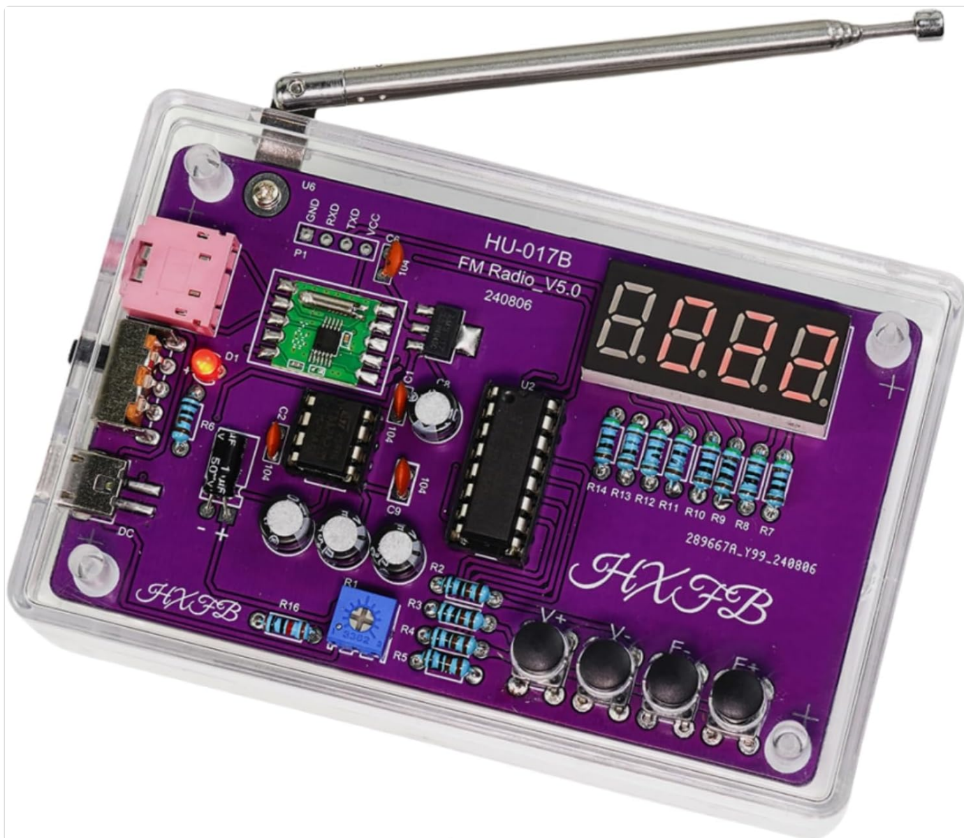
Figure 1: Assembled MUXWELL DIY FM Radio Kit.
