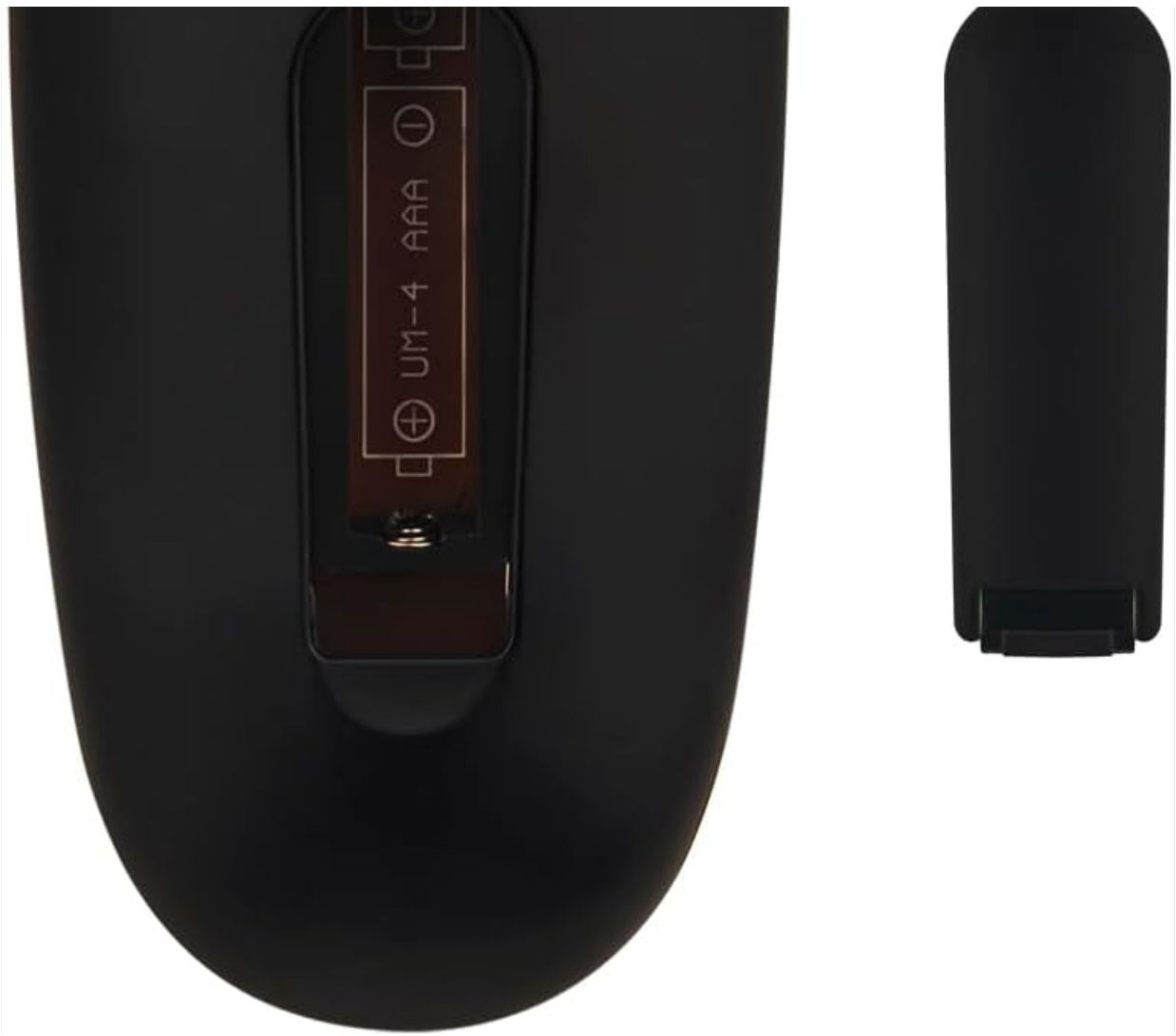
Figure 2: Back view of the remote control with the battery compartment open, illustrating the correct orientation for AAA battery insertion.
