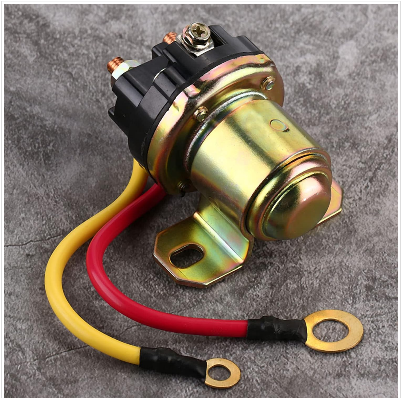
Image: A detailed view of the Sriya Starter Motor Solenoid Relay, highlighting the terminals for connection. Note the two smaller terminals for ground and ignition signal, and the two larger terminals for the main power supply to the starter.
