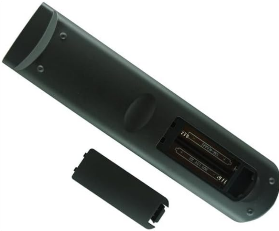
Figure 3.1: Battery compartment open, illustrating correct battery placement.
