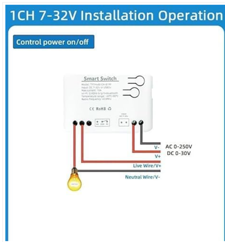
Image: Installation diagram illustrating how to connect the smart switch to control a light bulb, showing Live Wire/V+ and Neutral Wire/V- connections for the load, and AC 0-250V / DC 0-30V output.
