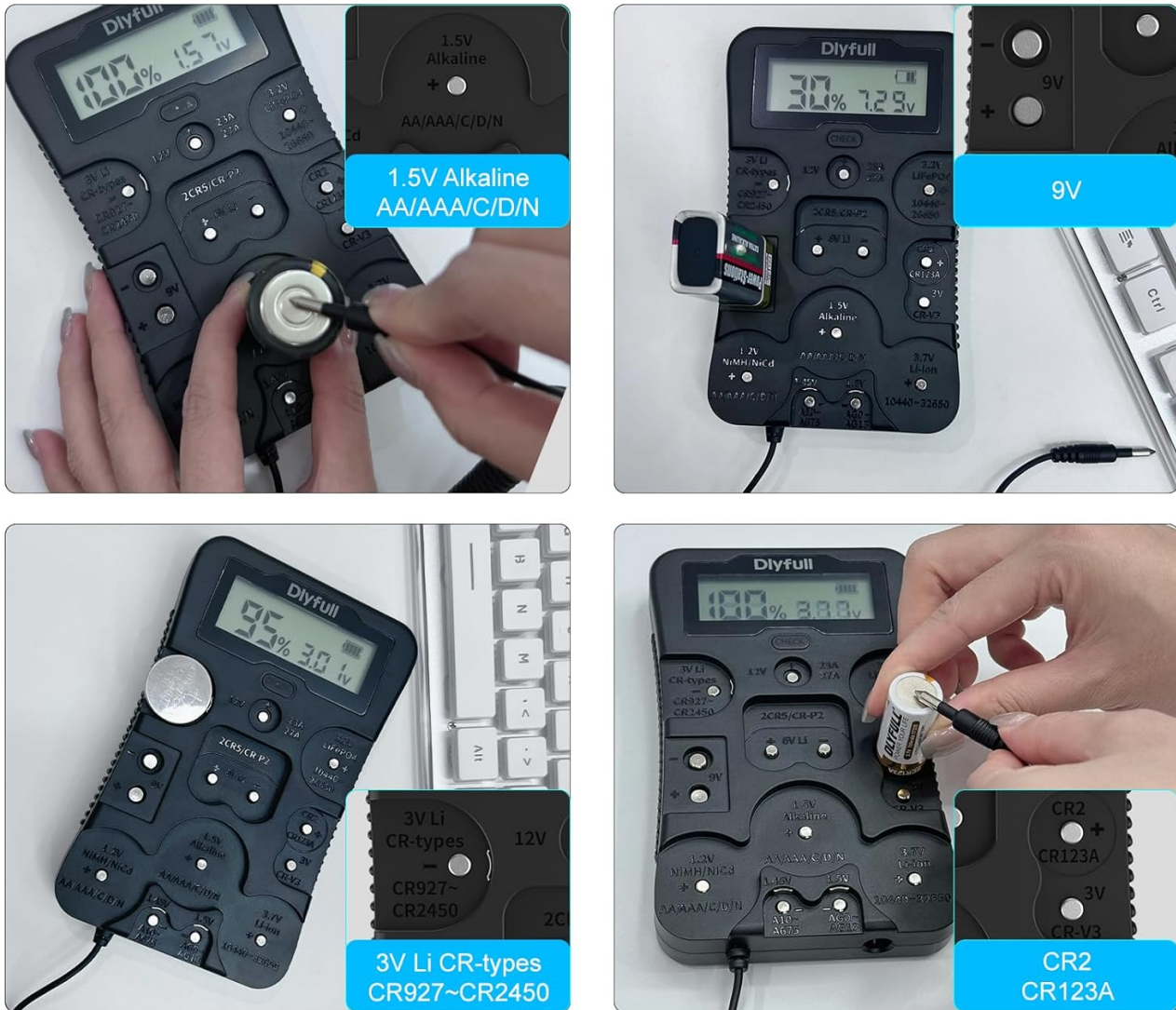
Figure 4.1: Demonstrations of testing various battery types (1.5V Alkaline, 9V, 3V Li CR-types, CR2/CR123A) using the Diyfull B4 Universal Battery Tester.
