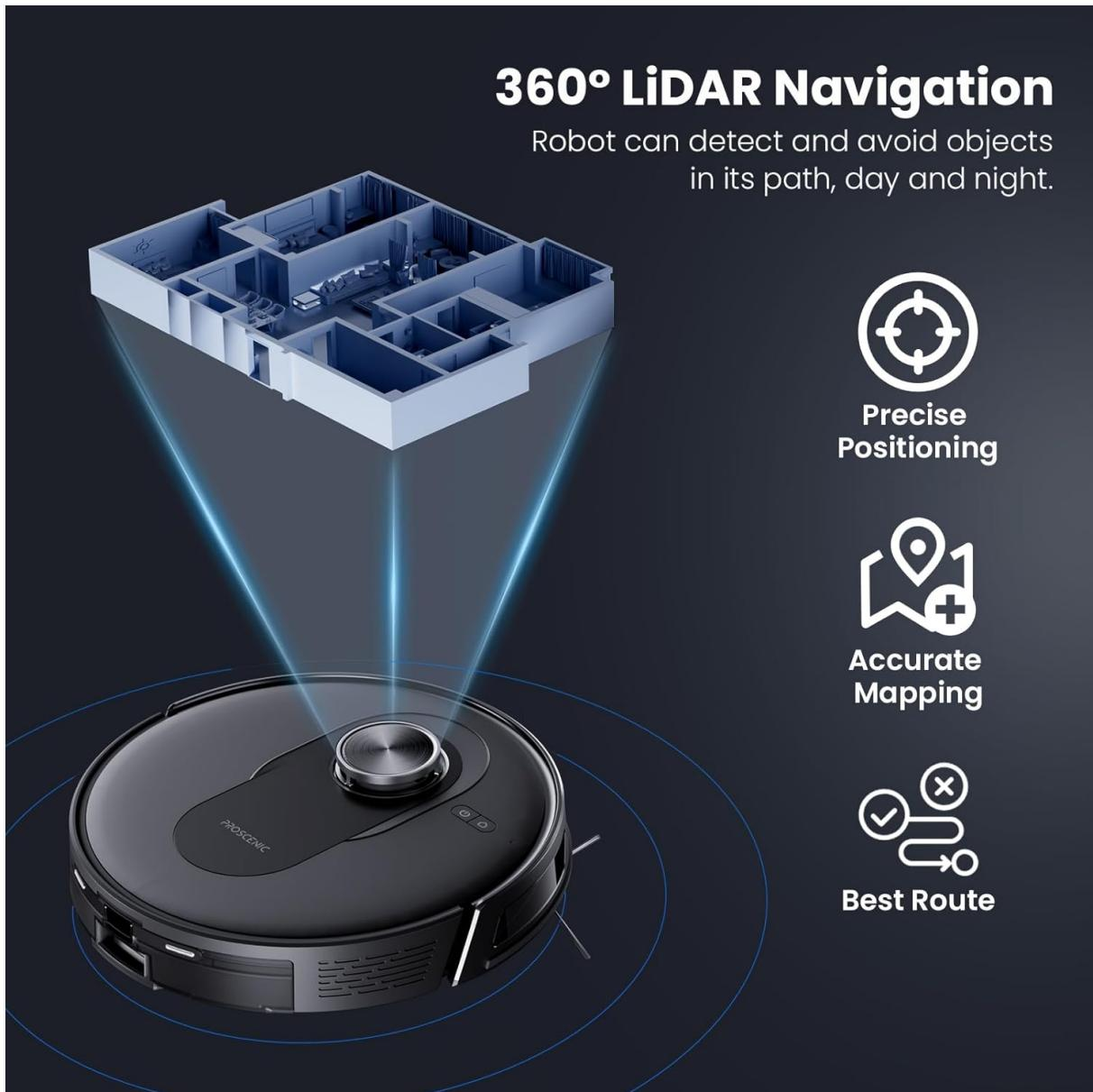
This image illustrates the 360° LiDAR navigation system of the Proscenic Q8. The robot uses laser technology to precisely map its environment, enabling accurate positioning, efficient mapping, and optimal route planning to avoid obstacles day and night.
