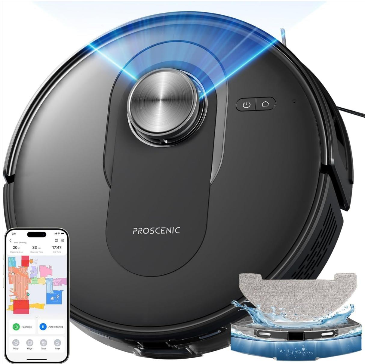
This image displays the Proscenic Q8 Robot Vacuum Cleaner from a top-down perspective, alongside its charging base and a detachable mopping module. The robot features a central LiDAR sensor for navigation, a power button, and a home button. The accompanying smartphone app interface is also shown, illustrating mapping and control functions.
