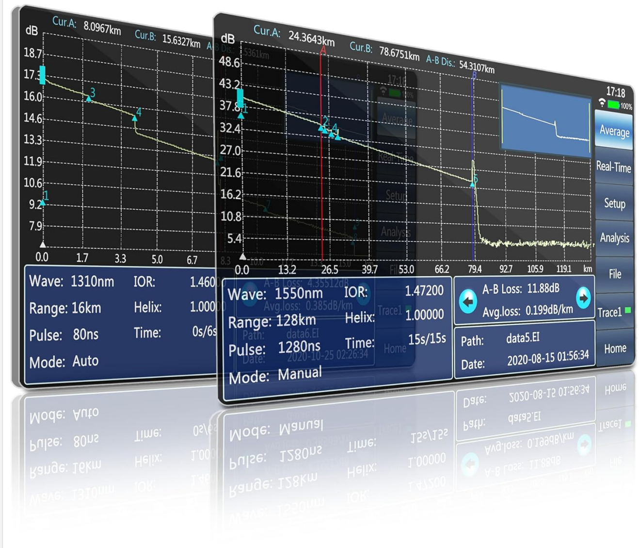
Figure 6.2: A side-by-side comparison of OTDR test curves for 1310nm and 1550nm wavelengths, demonstrating different measurement parameters and results.
