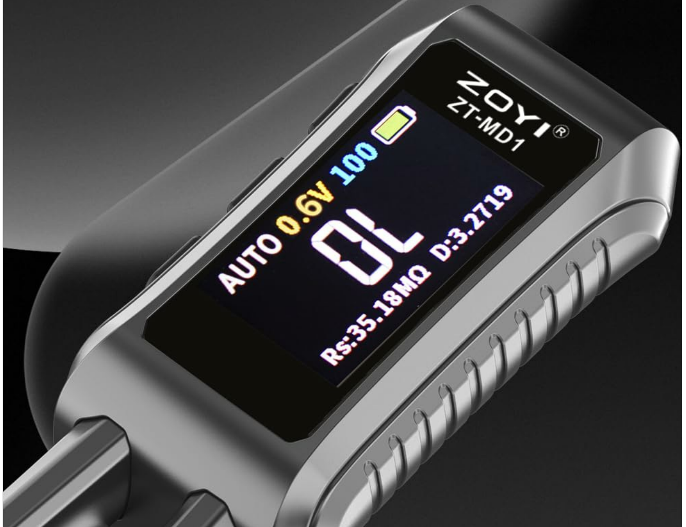
Image: Close-up view of the ZOYI ZT-MD1's 1.14-inch color OLED screen, demonstrating its clear, high-definition display.
