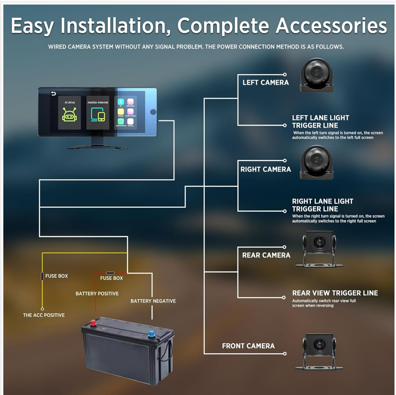
Image: Detailed wiring diagram illustrating how to connect the four cameras and the main monitor to the vehicle's power supply and trigger lines.
