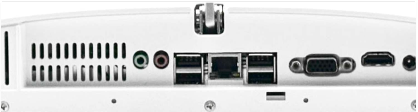
Rear connectivity ports including HDMI, VGA, USB, Ethernet, and audio jacks.
