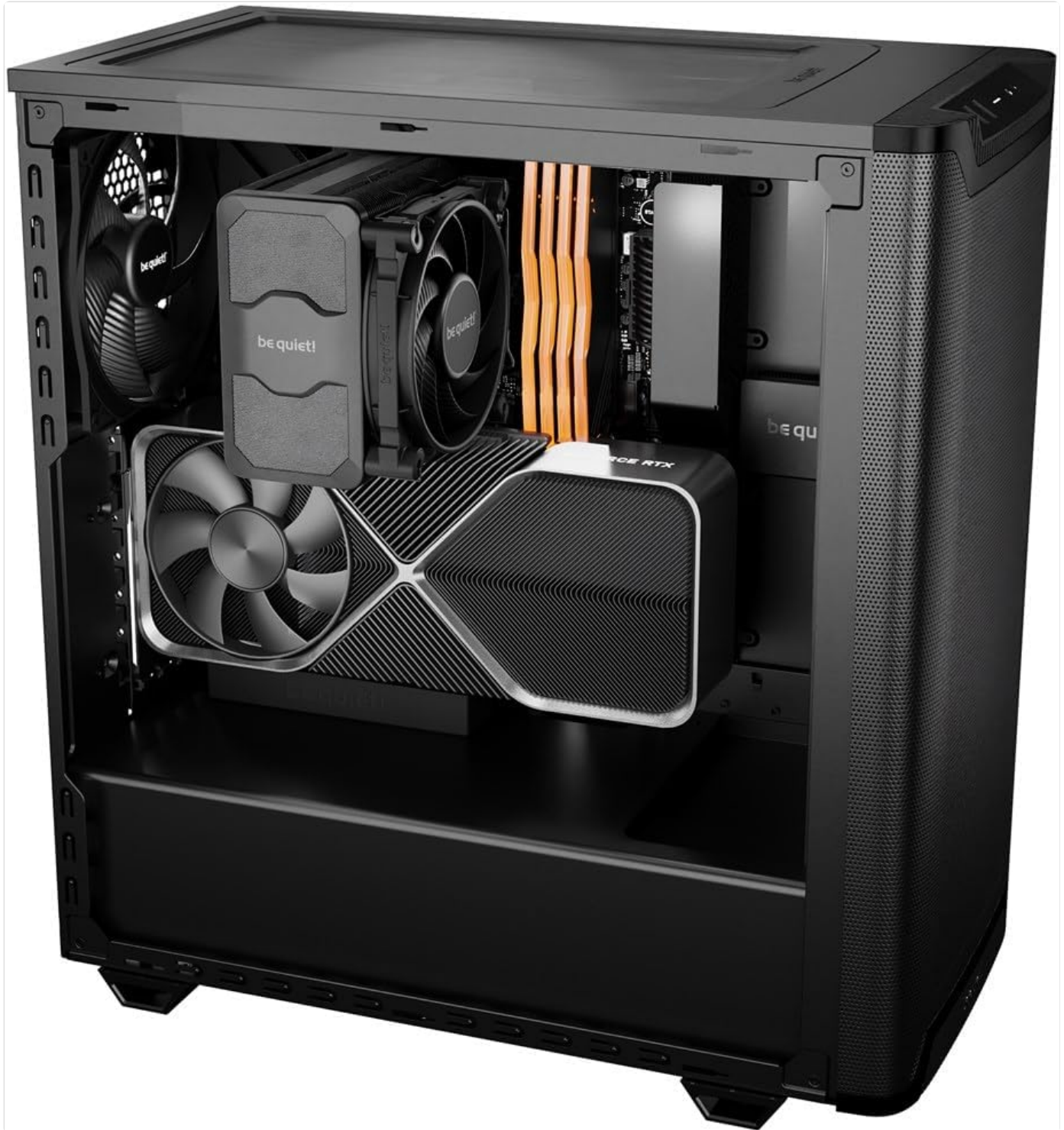
Figure 4.3: Example of a fully assembled system inside the case, showing component placement.
