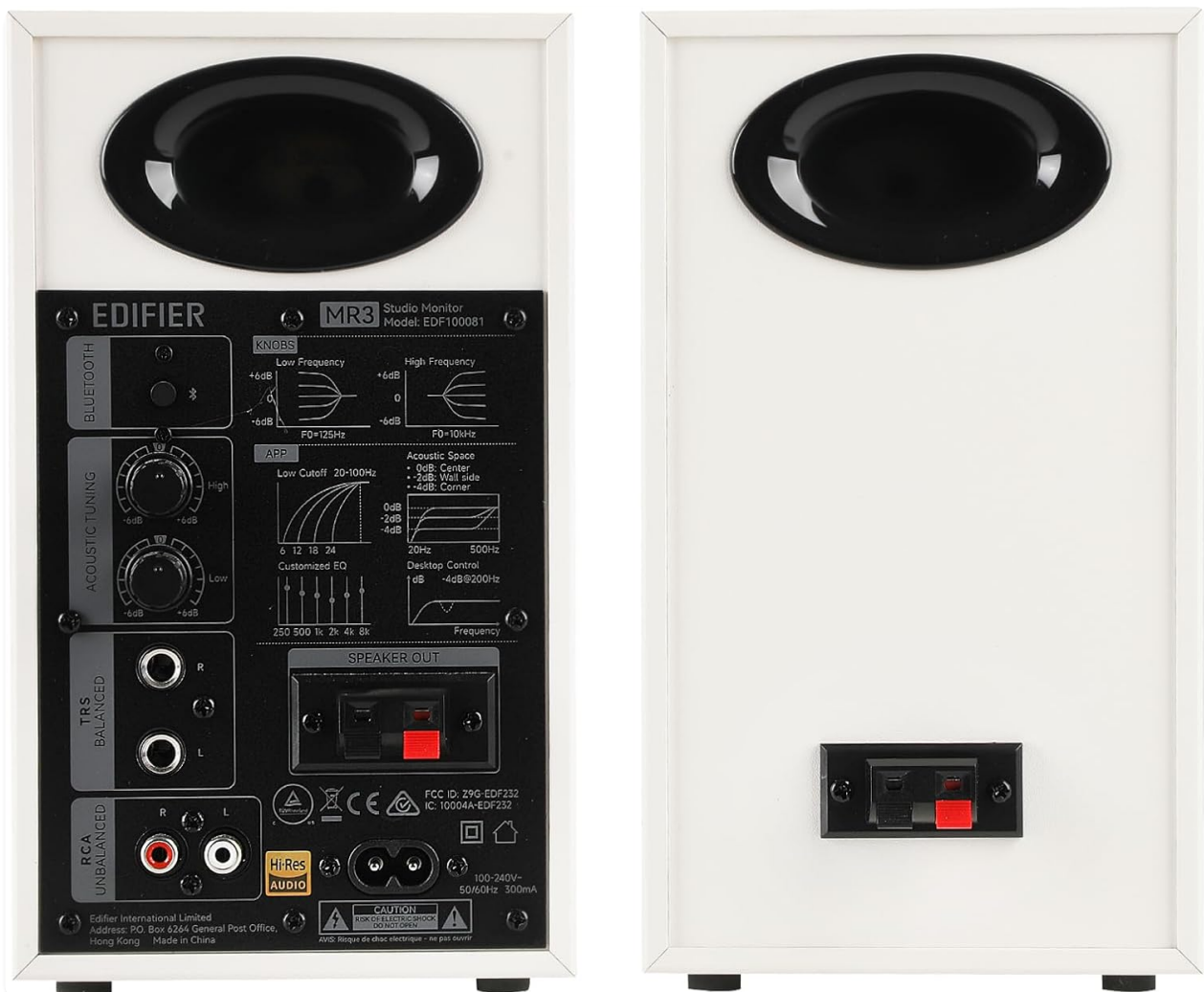
Image: Rear panel of the active Edifier MR3 speaker, detailing the various input ports and acoustic tuning controls.
