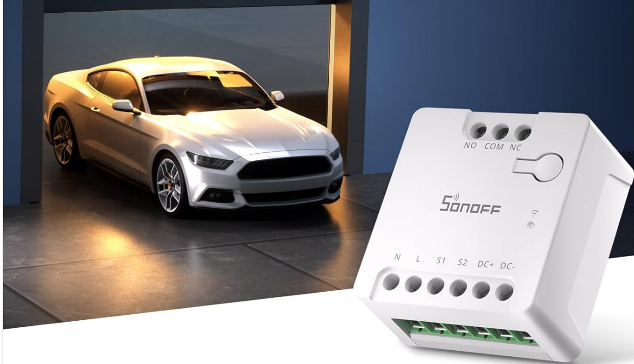
Figure 6.1: The MINI-D is compatible with various garage door systems, requiring an "Inching" setting for pulse-type motors.
