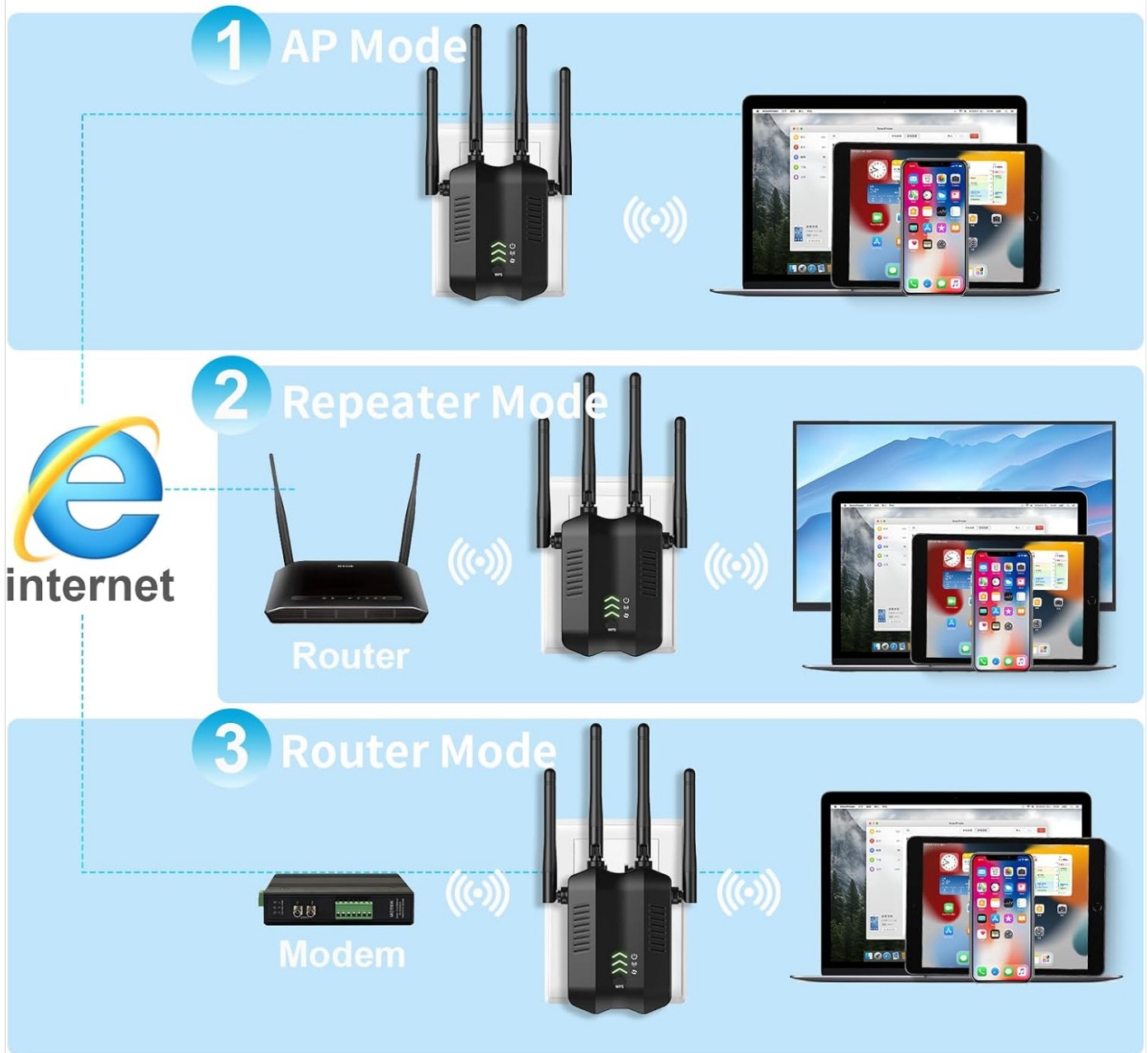
Figure 5.1: Overview of the 3-in-1 mode application, detailing AP Mode, Repeater Mode, and Router Mode connections.
