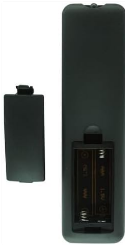
Image 2: Rear view of the remote control with the battery cover detached, revealing the two AAA battery slots. This illustrates the correct orientation for battery insertion.
