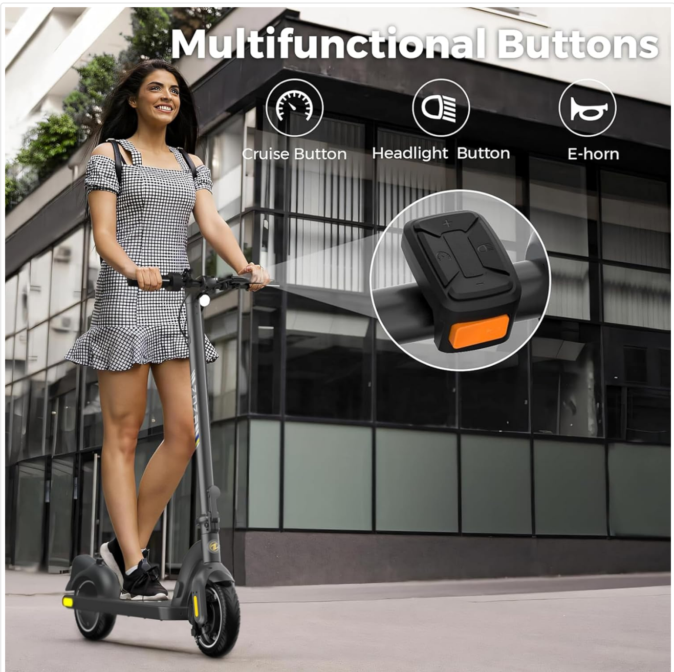
Figure 7.2: Multifunctional Buttons. This image details the buttons for cruise control, headlight, and E-horn on the left handlebar.
