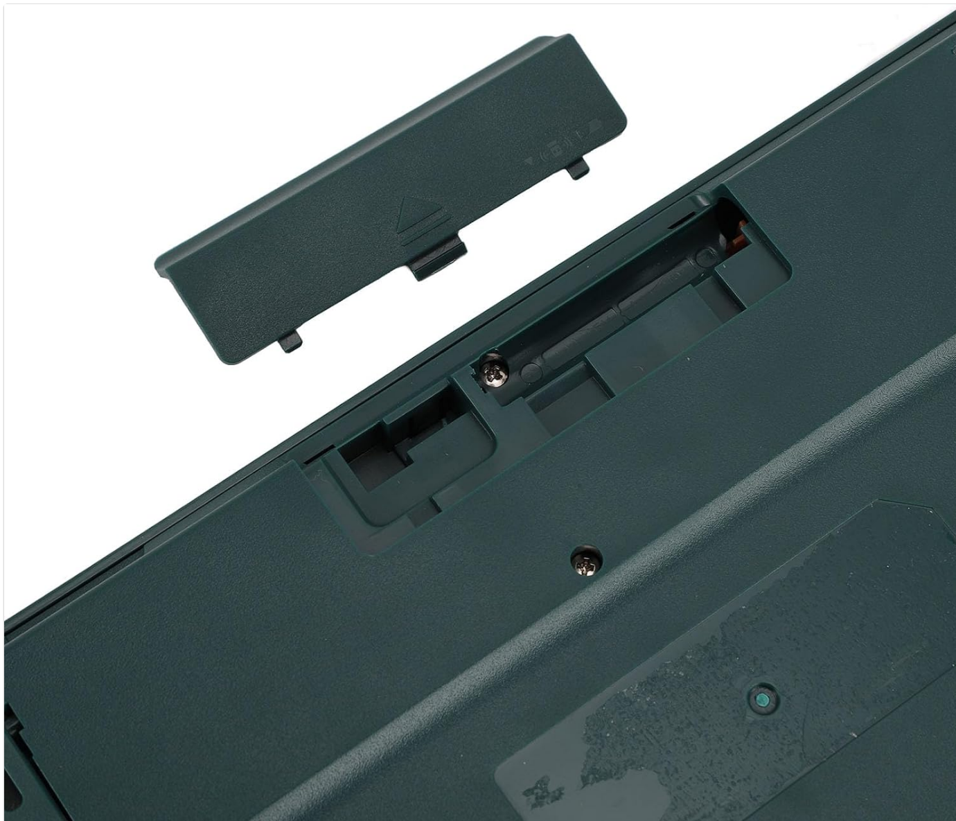
Image: A close-up view of the keyboard's underside, showing the open battery compartment where two AAA batteries are to be inserted.
