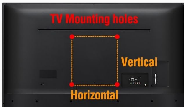
Figure 8: Detailed diagram of VESA mounting hole patterns.
