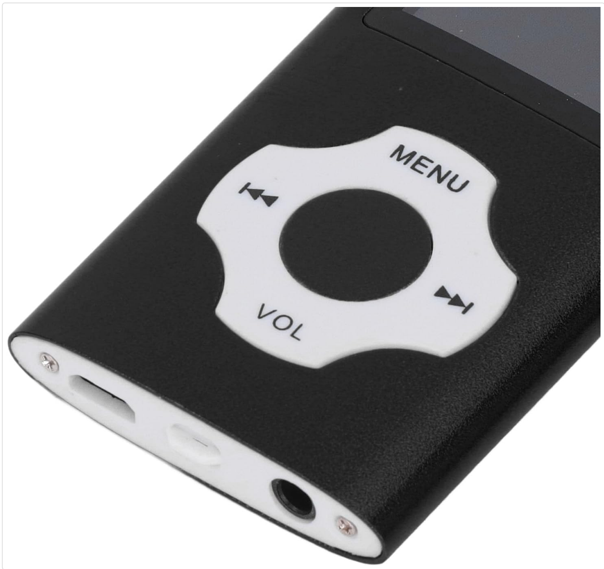
Image: Close-up view of the bottom edge of the player, highlighting the Mini USB port for charging and data transfer, and the 3.5mm headphone jack.
