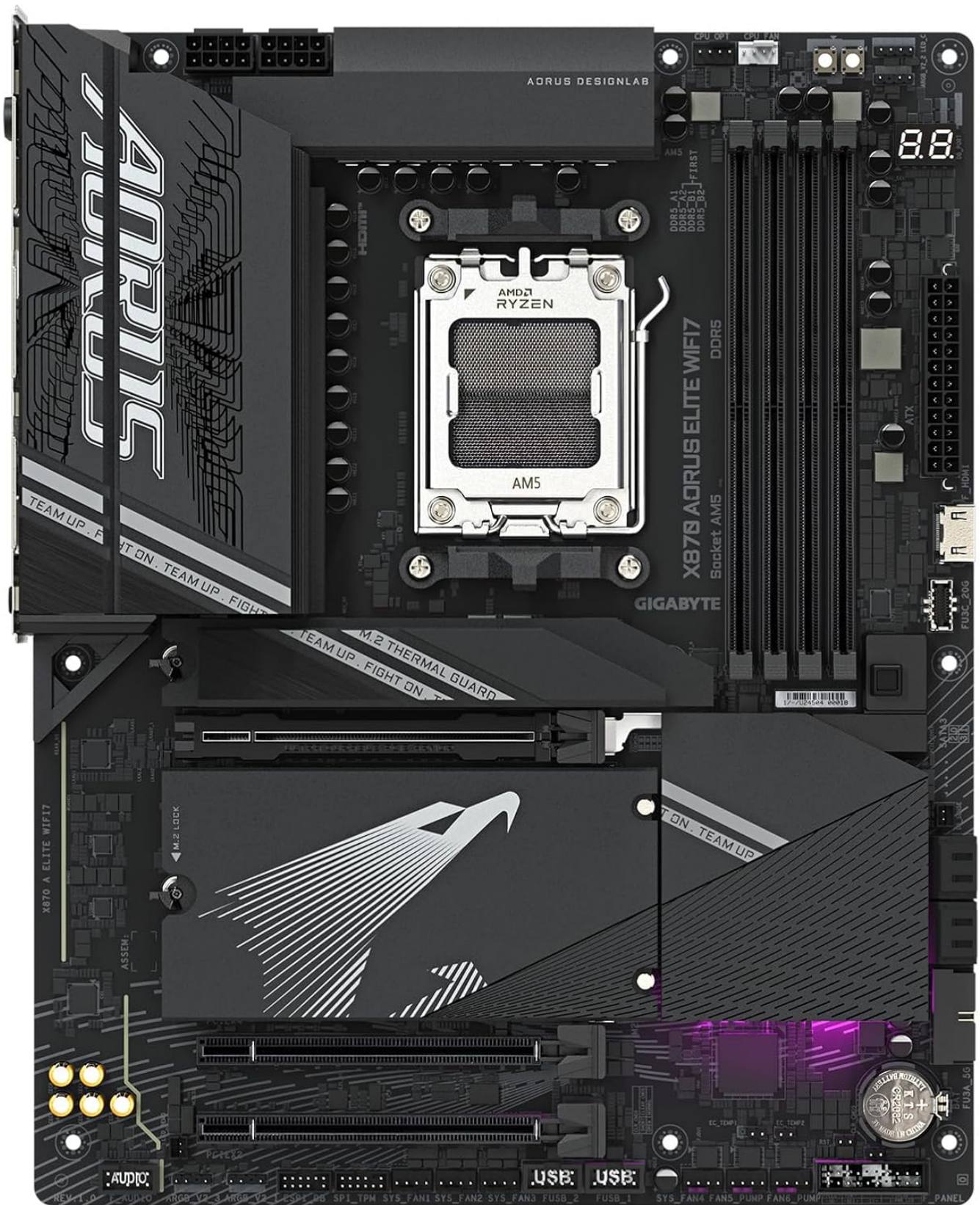
Figure 3.1: Detailed top-down view of the motherboard, showing CPU socket, DIMM slots, and M.2 slots.
