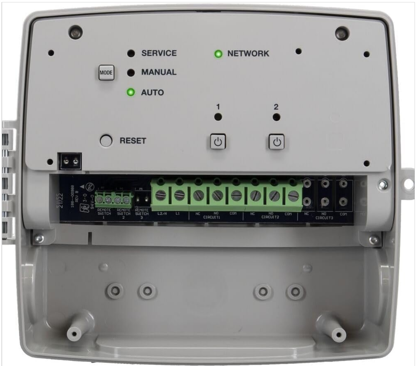
Figure 2: A detailed view of the ETW2CP's control panel. Visible elements include the MODE button, SERVICE, MANUAL, and AUTO indicator LEDs, NETWORK status LED, RESET button, and two circuit control buttons (1 and 2). Below these are the terminal blocks for power input (L2/H, L1, NC, NO, COM) and two independent circuits (CIRCUIT 1, CIRCUIT 2).
