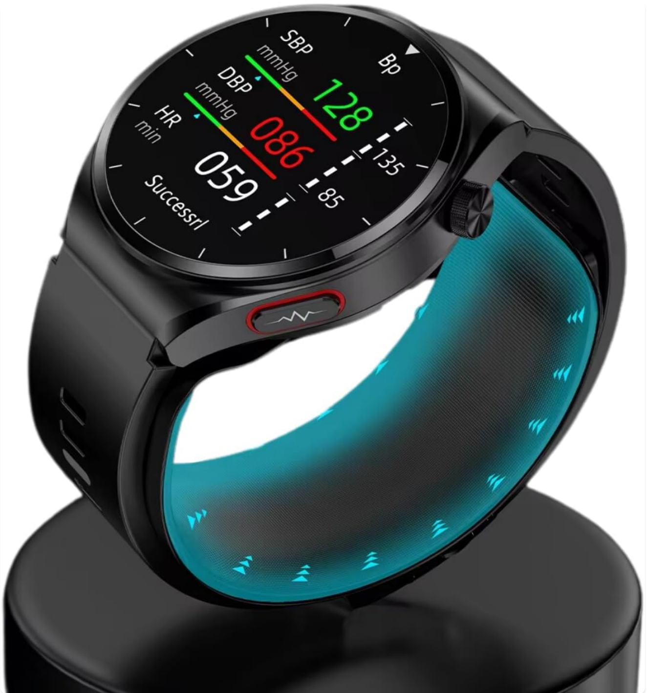
Figure 5: Heart Rate and Blood Pressure Display. This image shows the watch displaying heart rate (HR) and blood pressure (BP) readings, indicating successful measurement.
