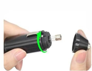
Figure 6.1: Visual guide for replacing the fuse within the car DC adapter's cigarette lighter plug. It shows unscrewing the tip, removing the fuse, and reassembling.
