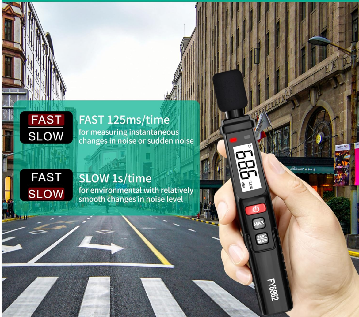
Image 4.5: Illustration of Fast and Slow measurement modes.
