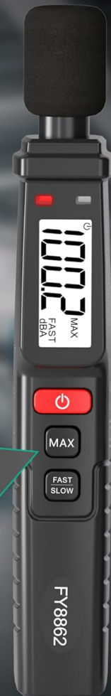
Image 4.6: The MAX Hold function for capturing peak sound levels.
