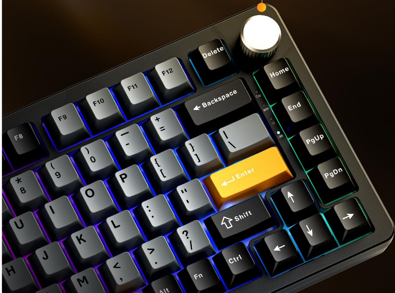
Figure 3.5: Multi-Function Knob. A close-up of the integrated knob, indicating its functions for volume control, media control, and programmability via web driver.
