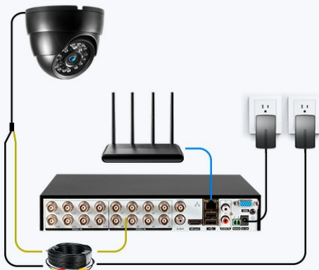
Image 4.7: A three-step guide for remote viewing: 1. Connect CCTV system to network, 2. Download free app (XMEye or ICSEE), 3. Enjoy live view.
