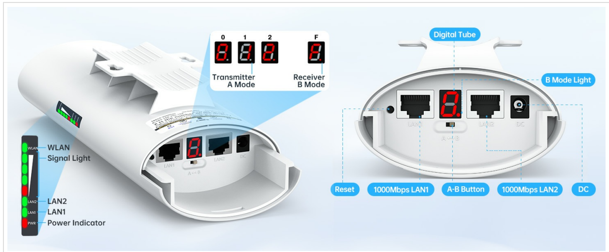
Figure 5: Visual guide for pairing Master (A) and Slave (B) bridges.
