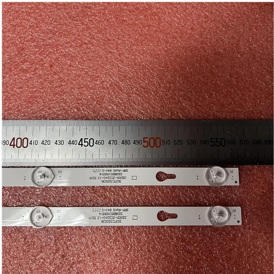
Image: The other end of the LED backlight strip, measured against a ruler, showing the final section up to 590mm, confirming the approximate 560mm total length.
