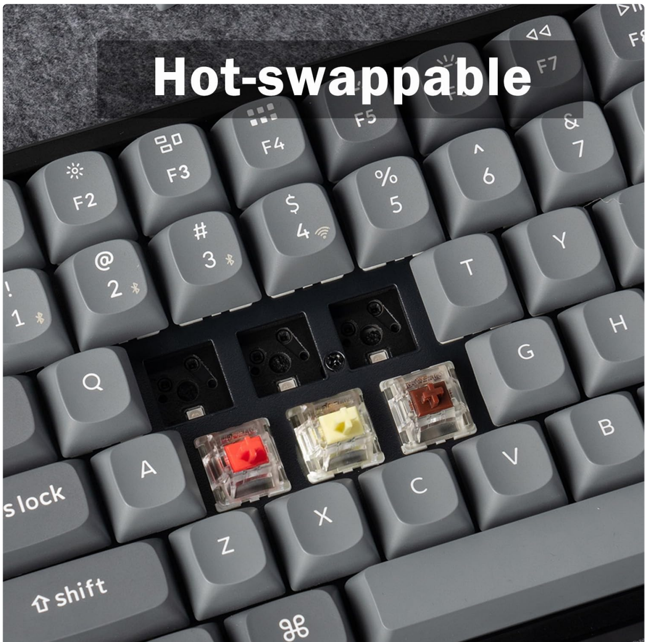
Figure 4.1: Close-up of hot-swappable switch sockets.
