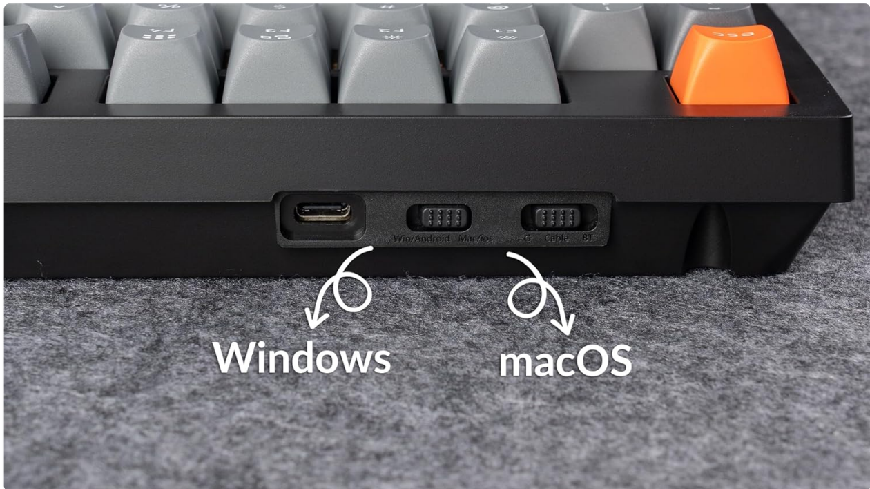
Figure 2.2: Switch for Windows/Android and macOS/iOS compatibility.
