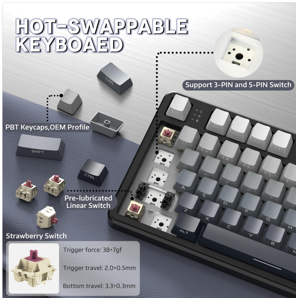
Image: Close-up view of the ATTACK SHARK X87's hot-swappable PCB, demonstrating how switches can be removed and replaced. It supports both 3-pin and 5-pin switches.
