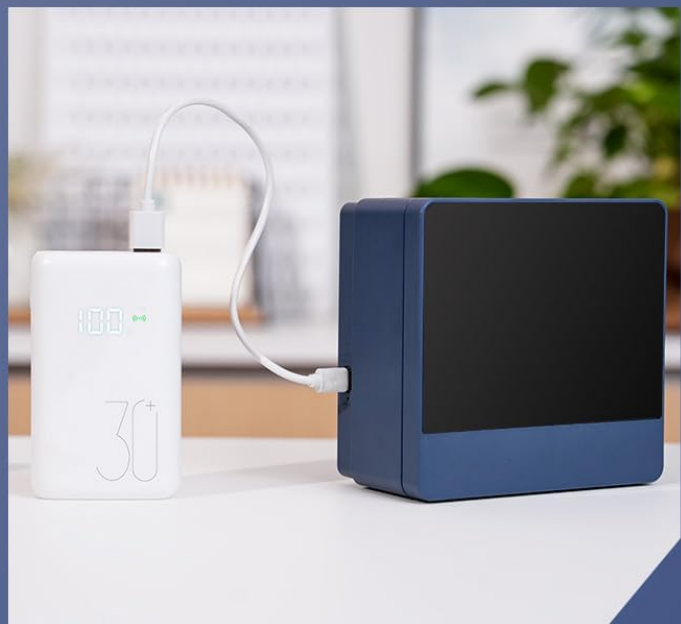
Image 2.1: Charging the P780BT Label Maker via USB Type-C.
