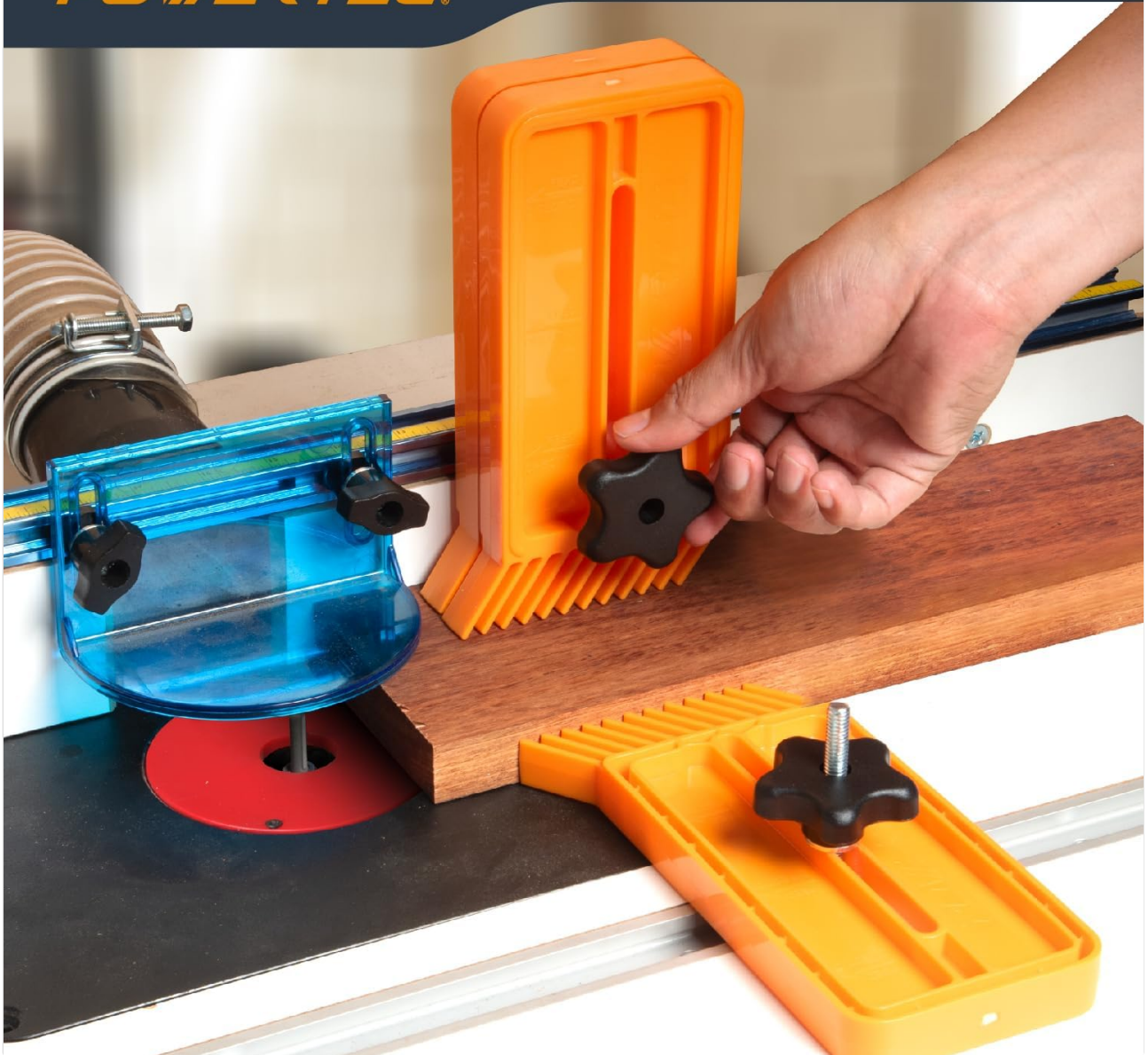
Figure 4: Featherboard setup on a router table.
