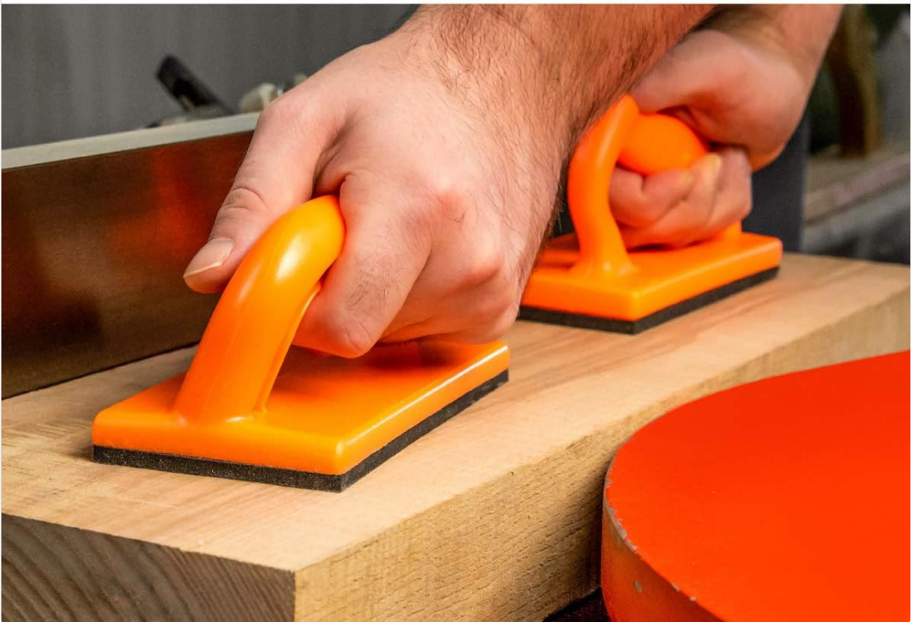
Figure 2: Push blocks protecting fingers and preventing kickback.
