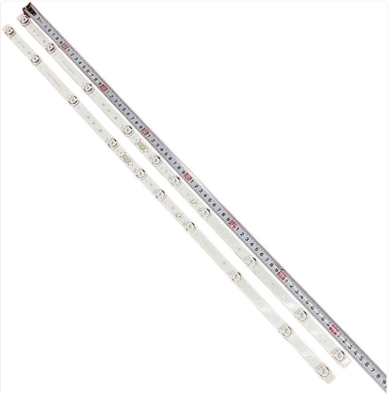
Image 2.1: Two TCETVMVXR LED backlight bars, each approximately 74.5 cm long, shown alongside a measuring tape for scale.
