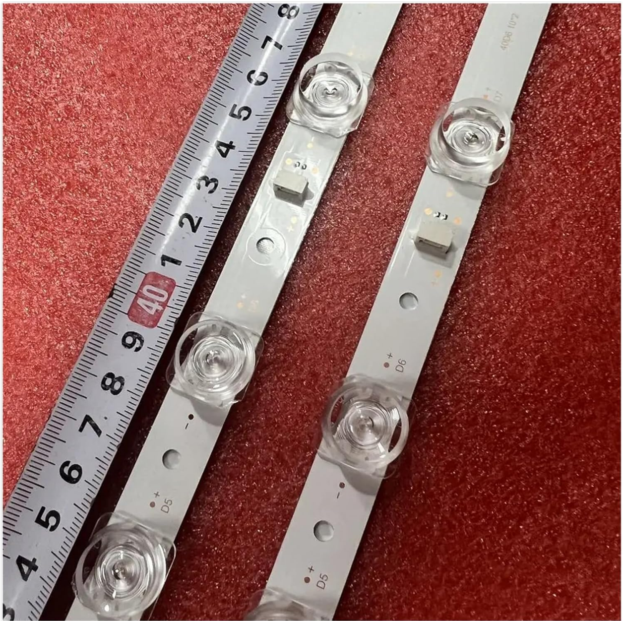
Image 2.2: Detailed view of an LED backlight bar, highlighting the individual LED components and a measuring tape indicating the 40 cm mark, confirming length specifications.
