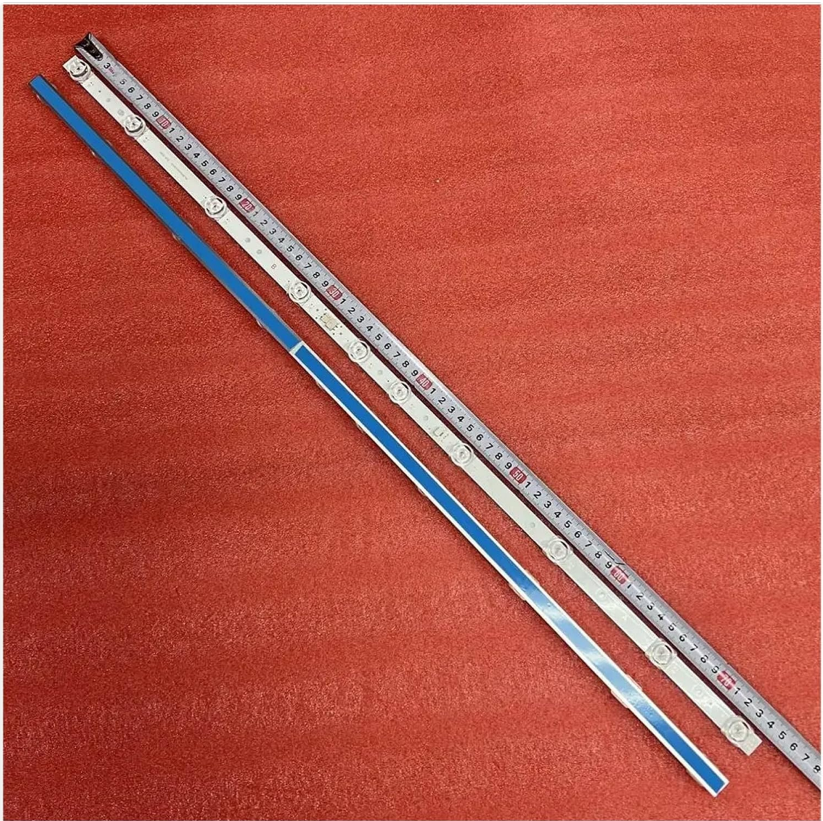
Image 4.1: The reverse side of two LED backlight bars, illustrating the adhesive backing used for secure installation within the television panel.
