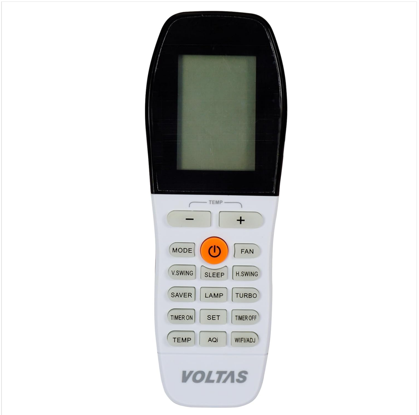
Image 1.3: Voltas AC Remote Control. This image displays the white remote control for the air conditioner, featuring various buttons for mode, fan speed, temperature adjustment, and special functions like 'Turbo' and 'Sleep'.
