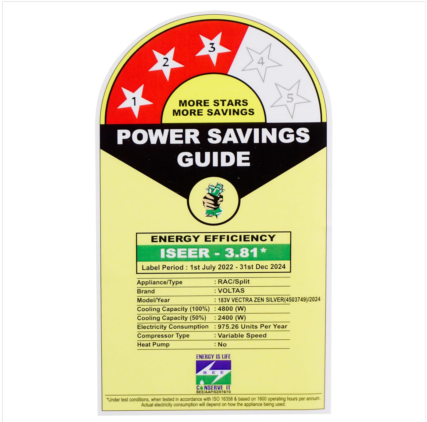
Image 7.1: Voltas AC Power Savings Guide Label. This image shows the energy efficiency label for the AC, indicating an ISEER of 3.81, 3-star rating, and annual energy consumption of 975.26 Units Per Year.
