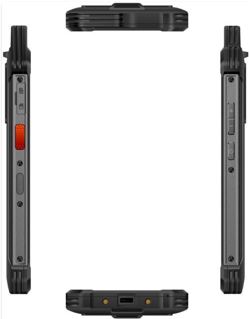
Figure 7: Various views of the UNIWA W999, highlighting its physical design and ports.
