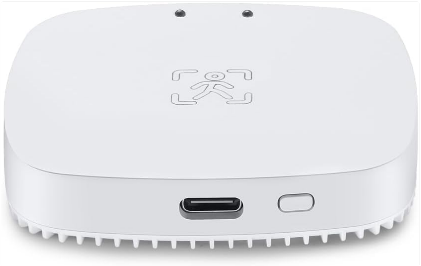
Figure 4.1: Close-up of the sensor's top, highlighting the USB-C power port and pairing button.
