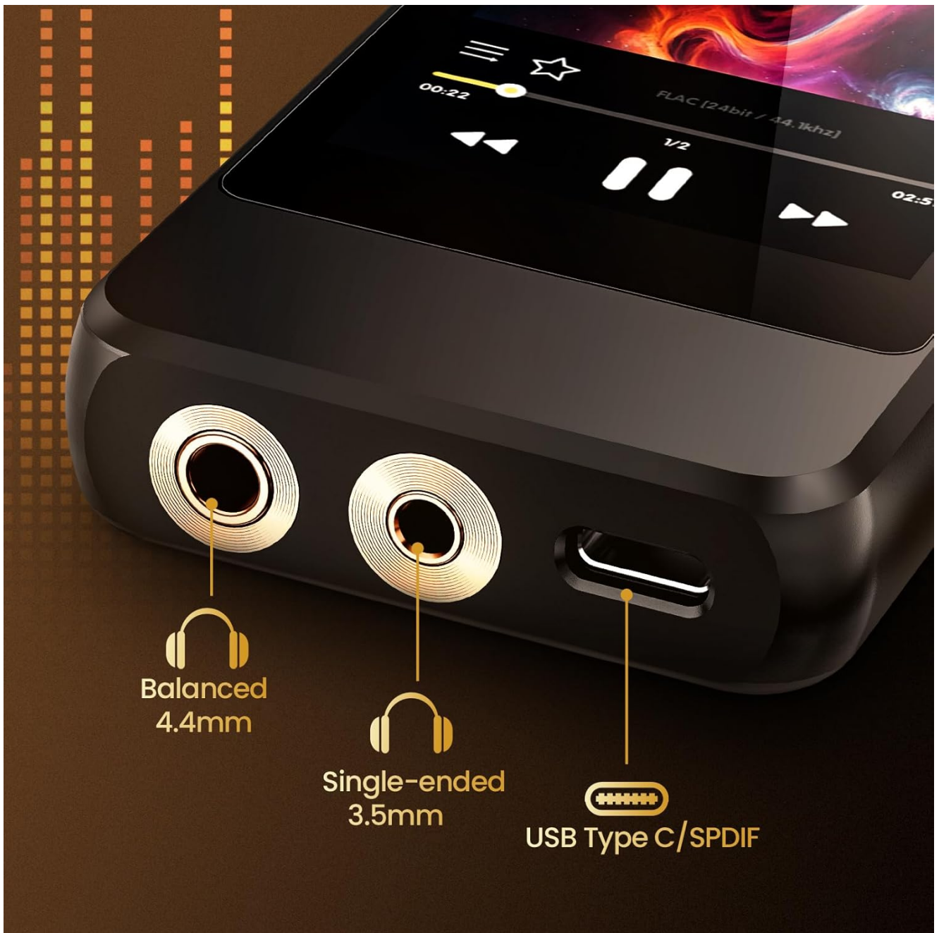
Image: Detailed view of the H20 Pro's audio output ports and USB-C port.
