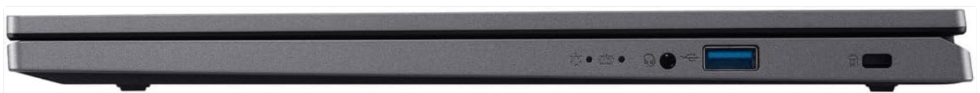
Image: Left side view of the Acer Aspire 5 laptop, displaying two USB 3.2 Gen 1 Type-A ports and the headphone/microphone combo jack.
