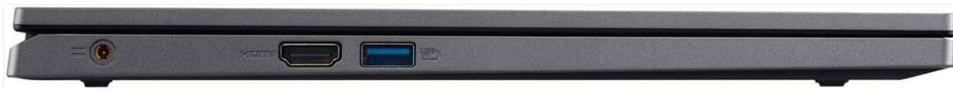
Image: Right side view of the Acer Aspire 5 laptop, highlighting the power input port, HDMI port, and a USB 3.2 Gen 1 Type-A port.
